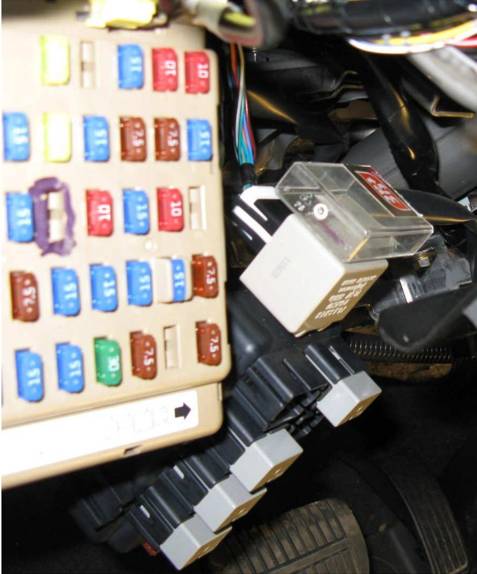
In order to best transmit the flasher vibrations, you need to use a brittle plastic such as the acrylic TicTac box or something similar. Don't use a bendable plastic like Nylon or PVC. Similarly, you should use a hard glue. I used CPVC plumbing solvent but epoxy should work ok. I would not recommend a flexible glue like Hotmelt or Silicone RTV.
