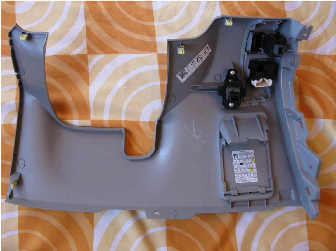
The flasher is located on the top of the relay block which is connected to the fuse box with two locking latches.
